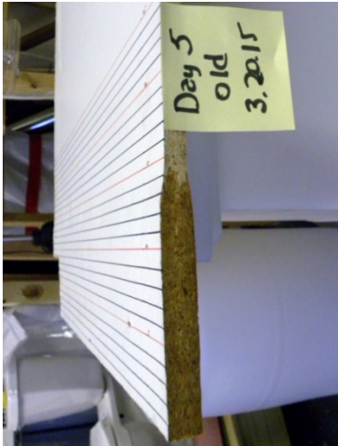
Photo 1. Thickness swell (1/2") is apparent after 5 days of continuous moisture exposure as identified by both sight and feel.
